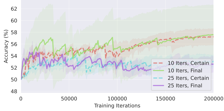
Figure 35 | Test accuracies for LSTM baselines, trained with either the certainty-based loss or the cross-entropy loss at the final internal tick. Both loss functions lead to unstable learning.
